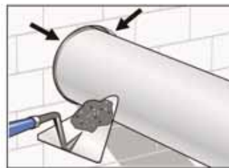
1-Seal cracks around the pipe using grout.
