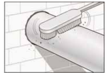
2-Clean the pipe before applying the fireproof sleeve.
